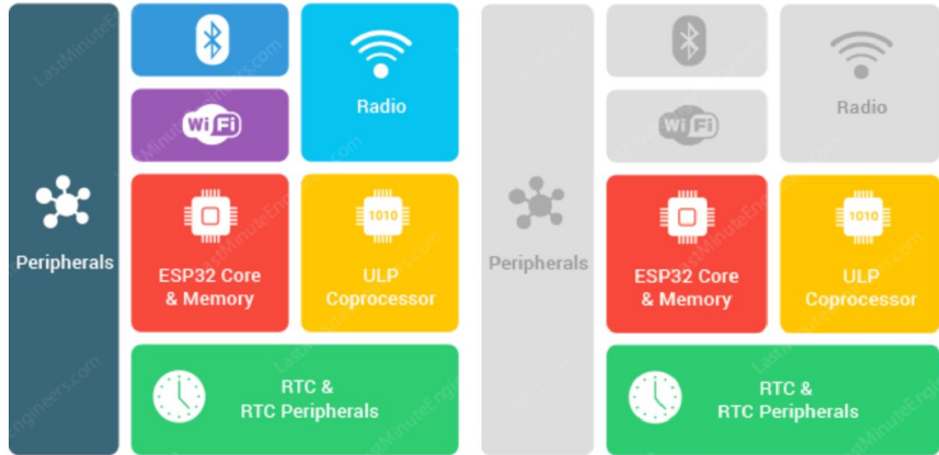
Figure 44: ESP32 Power Modes (Left:Active, Right:Modem Sleep) [66].
